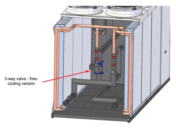
...which, after switching off the unit, can be accessed manually by removing the rear panel as show in the figure.
