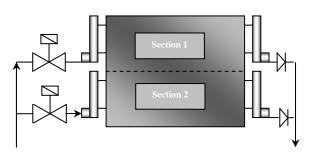
Indeed both sections of the coils are usually operative in the mechanical-only cooling mode, but when the Free-Cooling mode - therefore with T2 of the outside air below (T1-Delta T)°C - in the event of a simultaneous mechanical cooling request (integration), section 1 is excluded and ventilation runs at full speed whilst maintaining excellent control of the condensation pressure.
