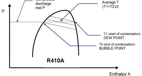
The difference between the Dew Point and Bubble Point is known as "GLIDE" and this is a characteristic property of refrigerant mixtures. If pure fluids are used, the phase change occurs at a constant T and thus the glide is equal to zero. If HFC R410A [ 50%-50% blend of R32 and R125] is used, the glide will be negligible (0.2°C) and the fluid can be considered like a pure fluid.
