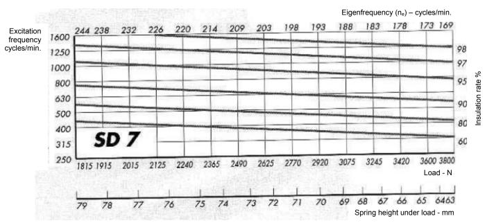
The ratings of the spring anti-vibration devices featured on the LCX Frame 1÷5 units are show in the diagram below:
