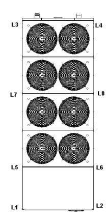
This drawing illustrates the points of the machine for which the **weights for the basic chiller and heat pump models** have been calculated. The values are shown in the following tables.
