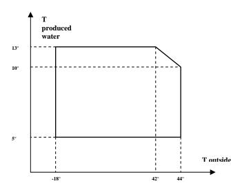
The lower limit is due to the limit of freezing temperature of glycol solutions with 35% of their weight made of glycol, the maximum admitted by the tightness of the pumps used.
