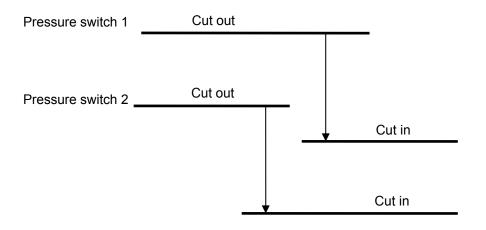
...where pressure switch 1 is set at the "PS" (maximum admissible pressure) of the system, while pressure switch 2 will have the setting =  $PS \times 0.9$  in accordance with the reference technical standard.
